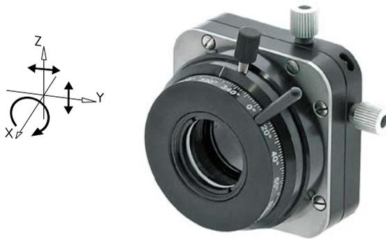
Two Axes Translation Polarizer Holder 840-0240 accepts optics of 25,4 mm diameter or with additionally provided adapter can accommodate smaller than 1" (25.4 mm) optics. The rotation position (X axis) is indicated on 360° angular scale with a gradation of 2°. The rotation platform has a removable rod that allows continuous 360° rotation without obscuring the aperture. This removable rod can be fitted into any of the four holes (10°, 100°, 290°, 280°) on the perimeter of rotation platform.
