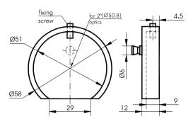
Connecting cone facilitates adjustment of the adapter. The cut-off side clears the edge of the optics for working with a beam very closely situated to another beam. Optics is firmly clutched by a stainless steel fixing screw and rests against the two contact lines formed at the cut-off side. The adapter is suitable for optical elements up to Ø50 mm (2 inch).
