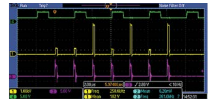
Example of driver operation. Green trace – modulated analog input signal, purple trace – trigger signal SYNC (single pulse control mode), yellow trace – HV pulse.
