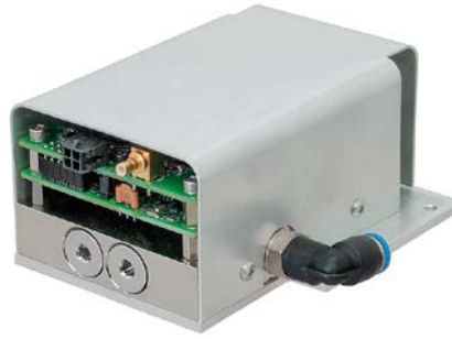
Standard of DP/DP-SP series Pockels cell driver
