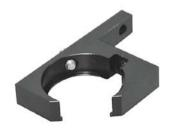
840-0100-A1 may be attached to the platform of 840-0102-T mount on any side. Optics is firmly held by a stainless steel fixing screw, and it rests against two contact lines – the edges of the cut-off corner. The frame doesn't obstruct the view. It allows to work with two beams going very close to each other.
