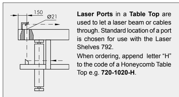
**Laser Ports** in a Table Top are used to let a laser beam or cables through. Standard location of a port is chosen for use with the Laser Shelves 792.
