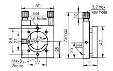
The Large Aperture Optical Mount 840-0150-T on its platform has Ø31.8 aperture and three M4 mounting holes. It is designed for precise orthogonal adjustment of mirrors.
