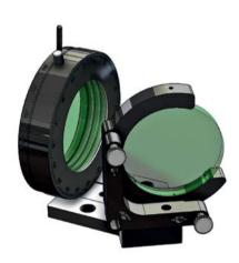
This variable attenuator/beamsplitter consists of Polarizer Holder 840-0180-A2 and Kinematic Mirror/Beamsplitter Mount 840-0056-13. UVFS Thin Film Brewster type polarizer Ø76.2 mm, which reflect s-polarized light while transmitting p-polarized light, is housed into Beamsplitter Mount 840-0056-13. A quartz Multi Order Half Waveplate Ø40 mm housed in rotating holder 840-0180-A2 and placed in the incident linearly polarized laser beam.
