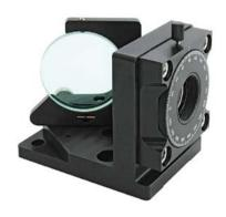
This variable attenuator/beamsplitter consists of Polarizer Holder 840-0190-01 and Kinematic Mirror/Beamsplitter Mount 840-0056-12. UVFS Thin Film Brewster type polarizer diameter 50.8 mm, which reflect s-polarized light while transmitting p-polarized light, is housed into Beamsplitter Mount 840-0056-12. A quartz Multi Order Half Waveplate diameter 25.4 mm housed in rotating holder 840-0190-01 and placed in the incident linearly polarized laser beam.
