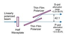
or their intensity ratio, can be controlled over a wide dynamic range. P-polarization could be selected for maximum transmission, or high-purity s-polarization could be reflected when maximum attenuation of the transmitted beam takes place. The holder 840-0197 allows to adjust angle of incidence of the Thin Film Brewster type polarizers by  $\pm 2^{\circ}$  and to get the maximum polarization contrast.
