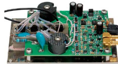
OEM version of DPS/DPD series driver with conductive pad. Suitable for repetition rate up to 50 kHz
