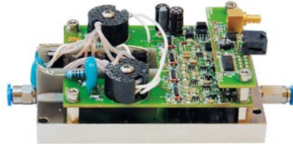
OEM version of DPS/DPD series driver with general purpose pad
