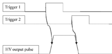
Fig. 1. Control timing charts for two-pulses controlled drivers
