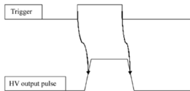
Fig. 2. Control timing charts for single pulse controlled drivers
