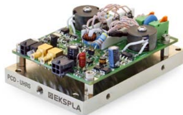
Fig. 16. OEM version of DP-SP series driver with general purpose pad
