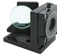
Variable Attenuator for femtosecond laser pulses 990-0072 page 5.19
