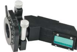
Variable Attenuators for linearly polarized laser beam 990-0070 page 5.14
