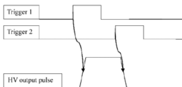
Fig. 1. Control timing charts for two-pulses controlled drivers
