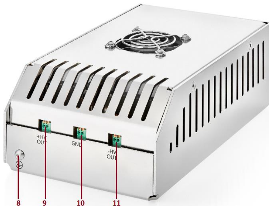
Figure 3. Rear controls of the HV power supply
