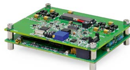
DQF-0.1-8 Pockels cell driver with integrated HV Power supply
