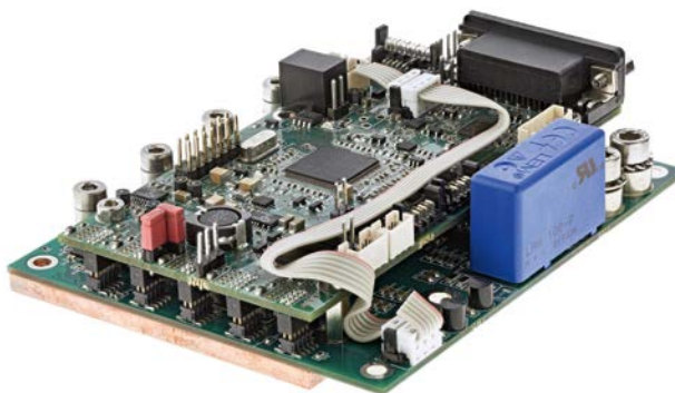
Conductive cooling driver version for CW operation
