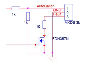
Figure 8. Fault output circuit
