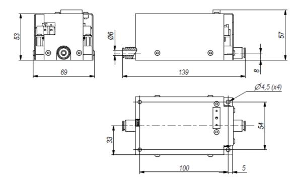
Figure 1. Outline drawing and dimensions of the driver
