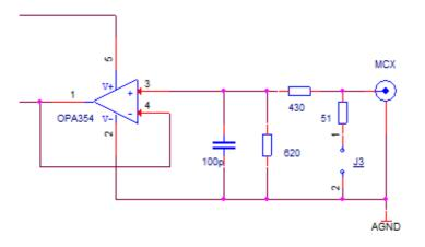
Figure 6. HV Control input circuit
