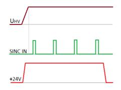
Incorrect driver operation. SYNC IN pulses appears before HV and 24V; SYNC IN pulses continues after 24V is switched off; HV supply gives an overshot.
