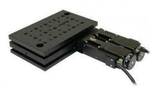
Multi-Axis Tilt Platform 6TP116 provides angular adjustment about two-axis - tilting and in-plane rotation. The mounting platform is rotated around kinematic pivot point by two micrometers.
