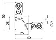
Prism Mount 840-01120-B provides basic mounting for prisms, beamsplitter, cubes and etc. Spring clamps 840-0111 series should be ordered seperately. This mount is metric compatible.
