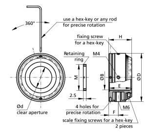
Polarizer Holder 840-0185 is an original mount with revolving conical angular scale on the face of the holder. This enables the user to set the current position on the scale to any chosen angle independently of the position of the holder.
