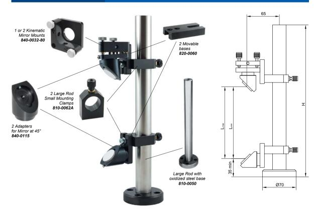
EKSMA OPTICS offers periscope on large rods assemblies that enables to adjust the height and change direction of a laser beam. The periscope assembly consists of two adapters for mirrors at 45° 840-0115 where mounted optics face each other. Mounting Clamps 810-0062A allows to adjust the distance between mirrors for a position needed.
