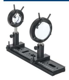
Simple lenses are subject to optical aberrations. In many cases these aberrations can be compensated for to a great extent by using a combination of simple lenses with complementary aberrations. A compound lens is a collection of simple lenses of different shapes and made of materials of different refractive indices, arranged one after the other with a common axis.
