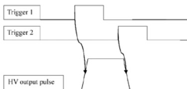
Fig. 1. Control timing charts for two-pulses controlled drivers
