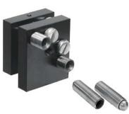
adjustment screws with a hexagonal head or a hexagonal keyhole. Miniature Precision Mirror Mount ensures precise angular adjustments of small optics about two orthogonal axes with 10 arcsec sensitivity. Mirror Mount is provided with M4 and M6 taped holes for mounting. These black anodized aluminium mirror mount is ideal for holding of 25 mm and smaller optic in tight spaces. A suffix to the unit code
