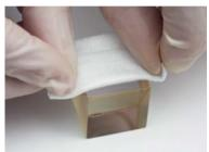
Always wear powder-free latex gloves or finger cots and handle component by the edges. Do not touch the surface of optical component with your fingertips. Avoid handling optics with metal instruments. Use delicate tweezers with soft tips for a small size components.
