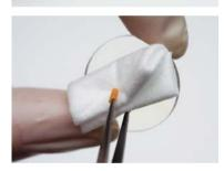
For the optical component cleaning apply a small drop of the cleaning solution on the top surface. Leave enough time for it to dissolve and float away any contaminating materials. But before the cleaner dries, gently wipe the surface with the highest quality lens cleaning tissue.
