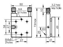
The Universal Mirror Mount/Platform 840-0140-T is suited for precise adjustment of standard mirrors which can be directly bound to it. The Mount may also be used in horizontal position as a tilt table. Then it can be used to align opto-mechanics around two axes.
