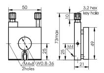
The Objective Mount of Side Control 840-0120-T has W0.8-36 mm aperture and is used for precise adjustment of standard microscope objective lenses and ensures low-cost positioning of a focus point. Also it can be used in the fiber optics.
