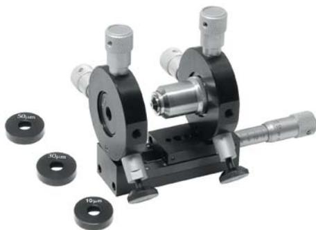
990-1000 with Precision Pinholes and Microscope Objectives
