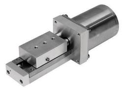
Vacuum compatible 961-0060V series stages are equipped with 10<sup>-6</sup> Torr vacuum compatible DC motor, all mechanical parts are lubricated with high vacuum compatible grease. Aluminum parts are not anodized.
