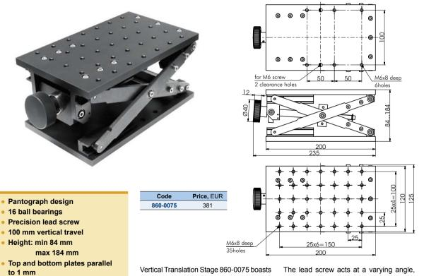
Vertical Translation Stage 860-0075 boasts our unique design. Being very compact, it provides smooth and stable adjustment of height. It has a large travel range, and it supports large loads. While moving the platform stays parallel to the base. The lead screw acts at a varying angle, so the resolution of the stage varies with position.
