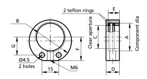
Optical Component Mounts 830-0037 can be used to hold round and thin optical elements of standard sizes. Mounts vary in dimensions so as to support diameters from 10 to 50 mm (0.5" to 2"). Original design allows to decrease the mount's dimensions and weight.
